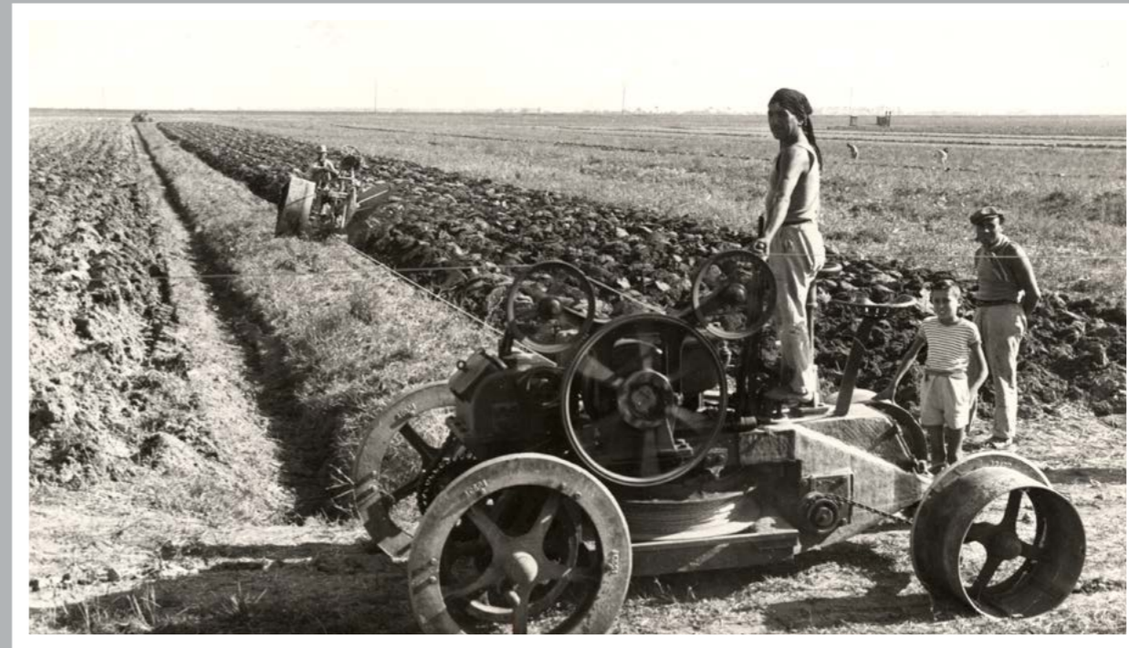
Alvaro Casadio, Funicular railway or Fowler plough: two-drives engines, Ravenna, 1940 Photographic Archive - Federation of the Cooperatives in the Province of Ravenna
